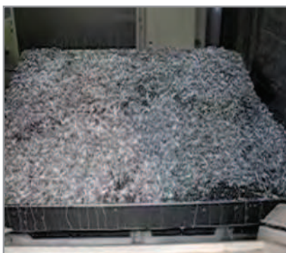
View into operating machining centre. Result: SAMURAI FASTAF proves reliable even with large chip volumes.
